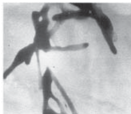
Fig.4. TEM Image of J aggregate of H_2TPPS_4^{4-}
